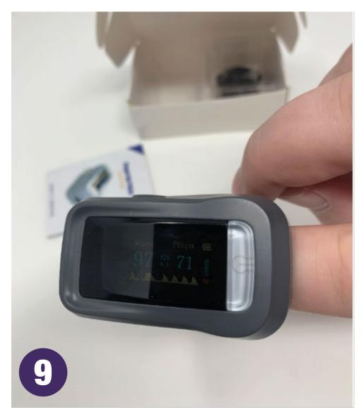
Reading will be displayed – oxygen levels to the left and pulse rate to the right Readings can change as live oxygen levels & pulse rate is continuously being monitored
